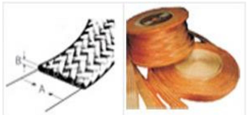
Braids made of many copper wires are also sometimes used for flexible electrical connections between large components. The numerous smaller wires comprising the braid are much more resistant to breaking under repeated motion and vibration than is a cable of larger wires.
